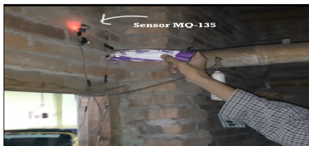
Fig. 17. MQ-135 sensor test with smoke
