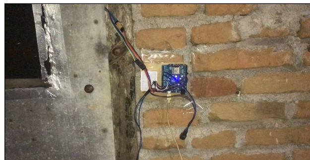
Fig. 18. The test of the MQ-135 sensor on the tobacco oven that are on.
